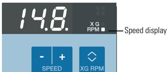
2. When the upper indicator is lit the display shows the RCF value. Press the
