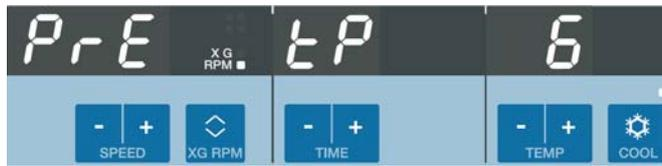
2. Enter the desired value by pressing the key
